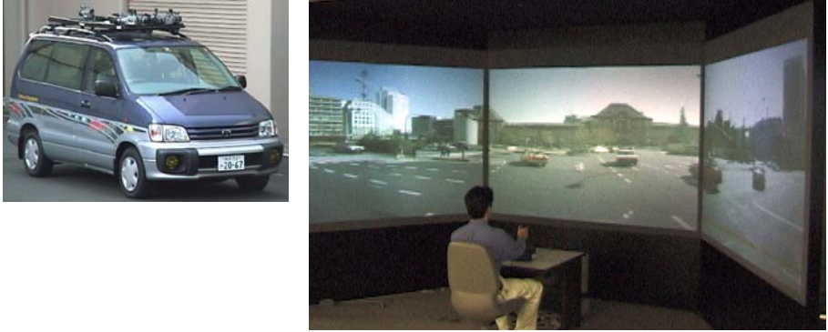
Fig. 7. “Cyber-city Walker” employed IBR technique to generate realistic street scenes. Image capturing car equipped with multi cameras is shown in the left.
